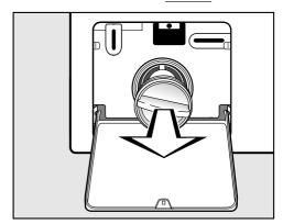
■ Remove the drain filter completely.
